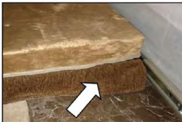
**Step 12** - Front bed – pull the outside tent flap underneath the bed and attach to the Velcro under the bed. Repeat for the rear bed.
