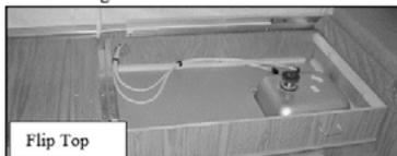
**Step 2** - Pull the fabric flaps loose covering the 4 lifter posts and tuck them behind the metal posts. Unsnap the two metal safety covers (on opposite corners) from the lifter posts (A), and place them together; store them under the front bed mat.
