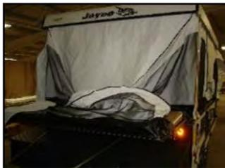
**Step 14** - Slowly begin to lower the roof. Stop periodically to insure the tent material is tucked inside the unit. Make sure the green cables are not tangled up on the lifter posts. Continue cranking the roof down until it is completely closed.
