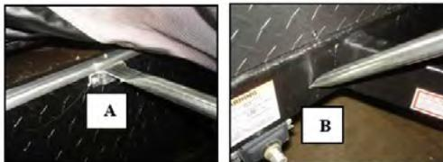
Hinged braces installed on the front of the RV.
