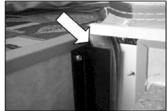
**Step 7** - Locate the bed bow braces under the front and rear bed mats. These braces have a large loop at one end and a small claw clamp on the straight end.
