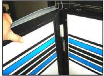
**Step 2** - The standard door is stored underneath the rear sliding bed. The hinges slide onto pins under the bed (A). The door pivots under the bed (B) and is held in place with a fabric strap.
