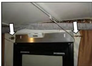
**Step 6** - On the outside of the door; secure the Velcro of the tent to the Velcro on the door. Make sure the tent portion does **NOT** overlap the hinges or the gap in the door frame. This can damage the door when opened. The latch side of the door should be done in a similar manner. Do **NOT** overlap the tent beyond the door frame edge.
