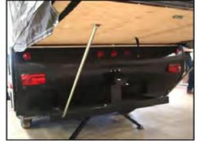
**Step 6** - If your model is equipped with a slideout, make sure the seal on the interior makes contact with the bracket on the slideout (arrow). The slideout should already be pulled out in order to slide the beds out (see **Step 4**).
