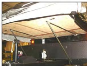
Install the (hinged) brace ends into the brackets (C) located under both beds (D). A second person lifting the bed will make it easier to insert brace into the bracket.
