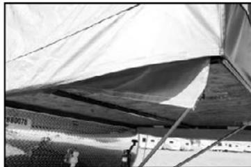
**Step 13** - If equipped with a slideout, Velcro the tent sides to the slideout. Adjust for water run-off.
