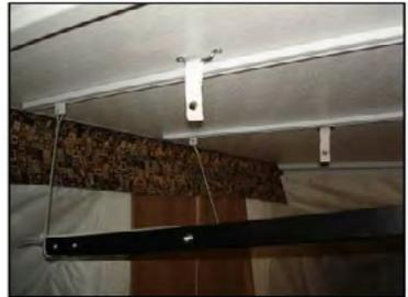
**Step 2 -** Turn the clip in the screen door bracket to release the bottom of the door. The clip will fit through the hole in the bracket. Lift the bottom of the door off of the rail and lower to the floor.
