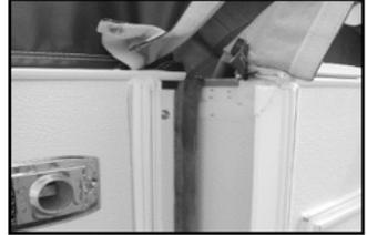
**Step 10** - Make sure the slideout tent (if so equipped) is pulled out and away from the unit. This will allow the front and rear beds to slide in without snagging the slideout tent.
