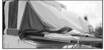
**Step 8** - Remove the standard entry door from under the rear bed and place it back into traveling position on the side of the unit. Slide the door onto the hinges on the side of the trailer.
