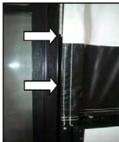
**Step 7** - Door installation is now complete. The door shades are built into the door. Press the gray tabs (arrows) at the top to slide the upper shade down. Press the gray tabs at the door latch and raise the bottom shade up.
