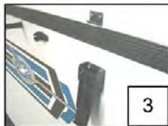
**Step 3** - The manual roof system is located on the tongue of the trailer. Attach the handle to the lift shaft and crank it until the roof is raised.
