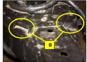
Repeat the process on the rear bed using the **shorter** braces. Make sure the bed is fully extended.
