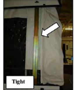
**Step 4** - If your model is equipped with a slideout, it must be pulled out (including tent) before extending the beds. This prevents the beds from catching on the slideout.
