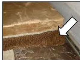
**Step 5** - Remove the bed bow braces from the bed bows on each bed and the ceiling brackets. Place the braces under the bed mattress. Place the sharp ends of the brace against the edge of the bed. If equipped with a slideout, remove the slideout bow brace and store it under the dinette table.
