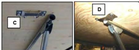
Repeat the process on the rear bed using the **shorter** braces. Make sure the bed is fully extended.
